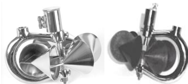
Рис. 10. Вертушка Прайса USGS TYPE AA-ICE MODEL 6240, USGS TYPE AA-ICE-P MODEL 6245 (Rickly Hydrological Company, США) (по [12; 19])
