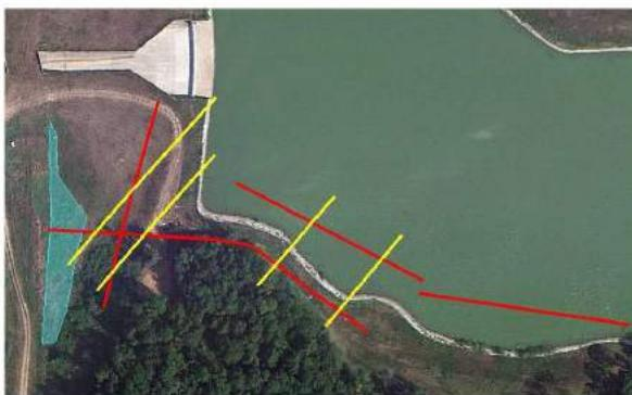
**Figure 8.** Interpreted solution-widened joint sets superposed on an aerial photograph of the study site (mark as yellow lines). ERT profile locations are marked as red lines. Lineaments orientation is southeast-northwest
